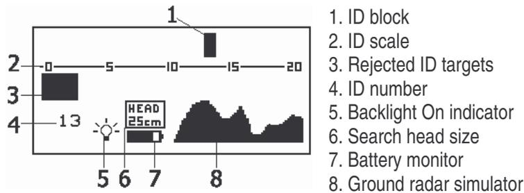
Ground radar simulator: this continuously scrolling radar is a view of the signal received by the **CSR1**. It can be used as an additional tool to analyse signals and it is also a useful pinpointing aid. It is visible in both full screen search mode and when the first level menus are displayed. The sensitivity of the radar display is controlled by the Pin Point Gain setting.
